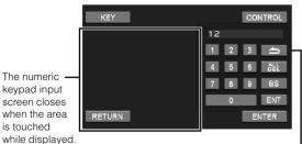
Touch [ 1] to close the numeric keypad input screen.
